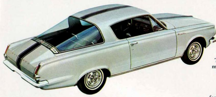
For the sporty set: A Commando 273-cu.-in. V-8 engine, "Rallye Pack" suspension (heavy-duty springs and sway bar), heavy-duty shocks. "Formula S" package: wide rim (14-in.) wheels, special wide tread tires, simulated bolt-on wheel covers, tachometer, plus "Rallye Pack", Commando 273-cu.-in. V-8 and heavy-duty shocks. (Note: "Formula S" options will be available in Fall, 1964.)
